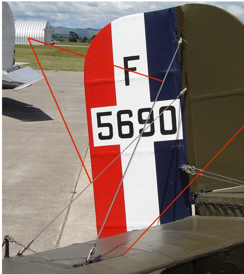
Extract from 'High in the Empty Blue' showing fin bowing during a spin or dive
