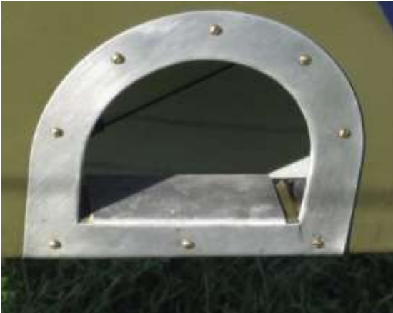
The photo at the left is of the step on the Sopwith Pup, built by 'Vintage Aviator Ltd' of New Zealand.
