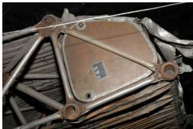
Gravity fuel tank in the upper wing.
