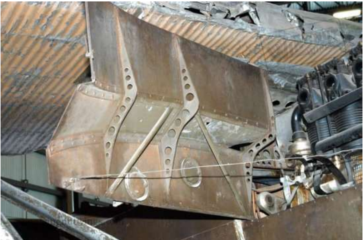
Right access door - forward, centre and rear bracing ribs
