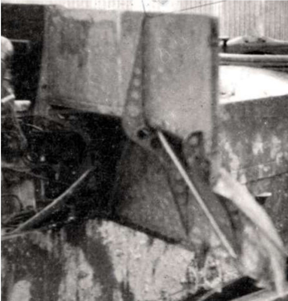
Left access door - front and forward bracing ribs
