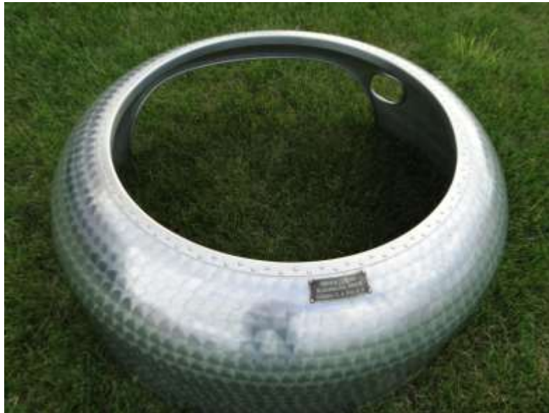
Modern example of a 'burnished' engine cowl.
