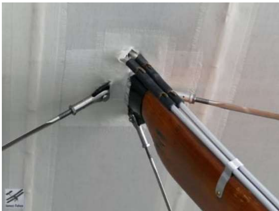
Actual end fittings for flying, landing and bracing wires.
