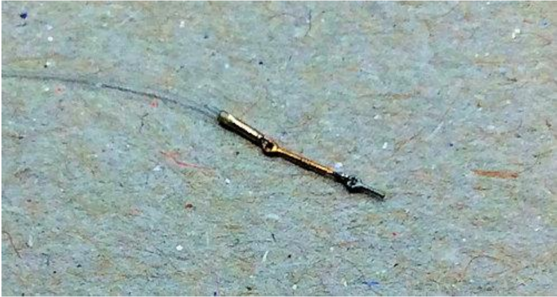
Example of a prepared cable or line (turnbuckle 'GasPatch' turnbuckle Type C)
