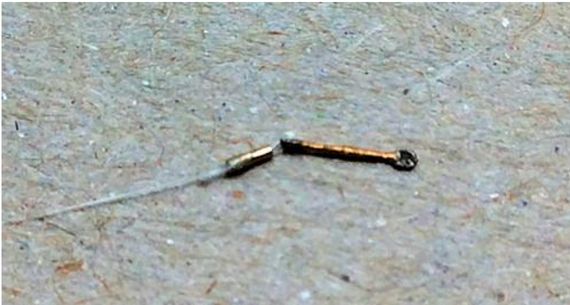
Example of a prepared cable or line (turnbuckle 'GasPatch' turnbuckle Type C)
