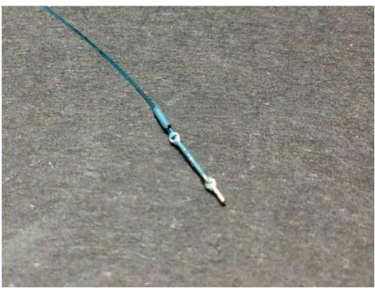
Example of Type A turnbuckle
