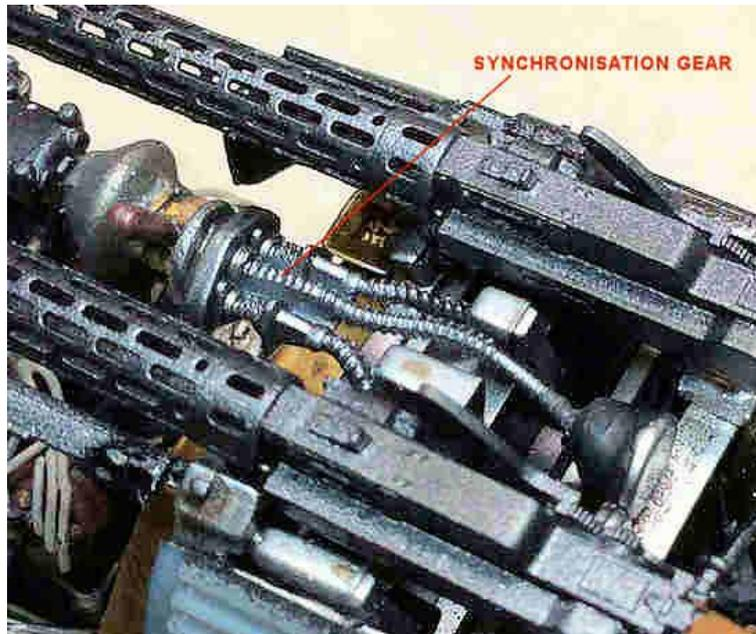
Test fit the inter panel between the two machine guns. Make sure the bottom edges of the panel fully contact the top edges of the fuselage upper side panels. Also make sure the panel locates without fouling either the weapons or the synchronisation gear.
