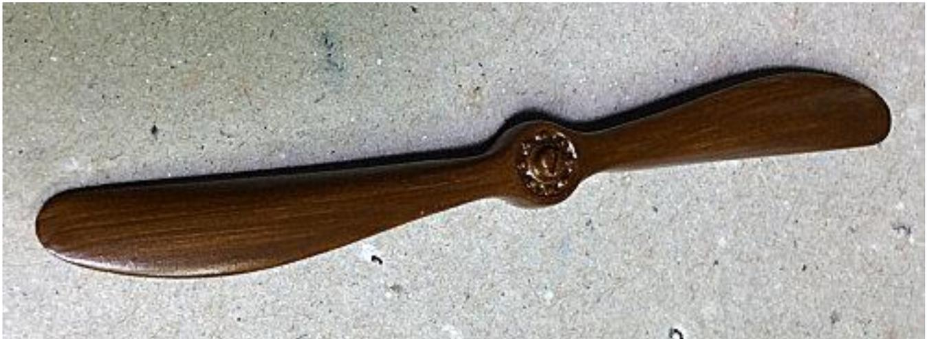
**NOTE:** *Once you are confident using this method of replicating wood finishes, you can vary both the colour of the acrylic base coat and tinting of the sealing coat, to replicate other types of wood used in aircraft construction.*
