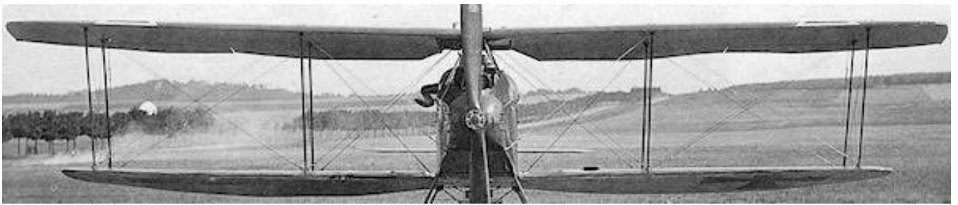
Wing 'washout' at trailing edges
