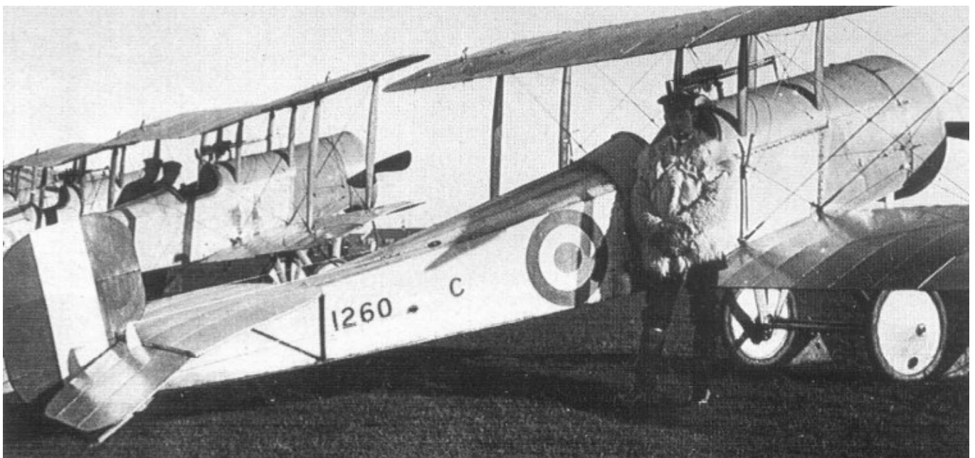
Scout 1260 with earlier fuselage mounted Lewis machine gun and full upper wing centre section
